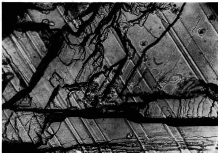
Fig. 5. Linear etch patterns on a calcium fluoride cleavage face ( \times 245 ).
